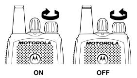
Turn the **On/Off/Volume** Control knob clockwise. If Volume Control knob power-up is successful. you will hear the Self-Test until you hear a click Pass Tone (  $\Box\Box$ and see the display icons light momentarily and the LED flash green.
