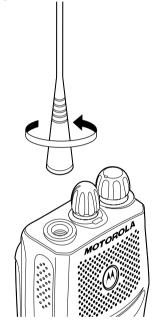
Turn the antenna clockwise to attach it.
