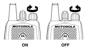
Turn the **On/Off/Volume** Control knob clockwise. If Volume Control knob power-up is successful. you will hear the Self-Test until you hear a click Pass Tone (  $\Box\Box$ and see the display icons light momentarily and the LED flash green.
