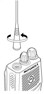
Turn the antenna clockwise to attach it.
