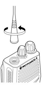
Turn the antenna clockwise to attach it.
